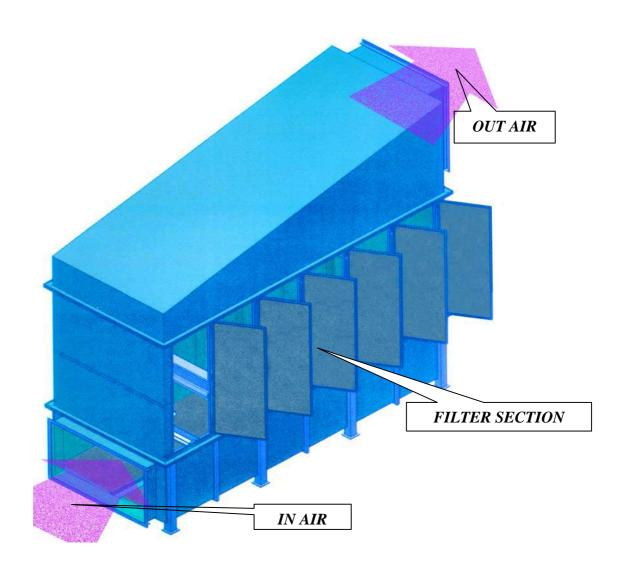
Particularly adapted for the collection and filtration of the air containing the suspended vapours of oil, diesel oil and other hydrocarbons.
